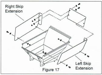
4. Align all panels and tighten hardware.
